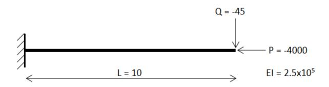
Shear deformations are ignored. Results are independent of cross section area; therefore any reasonable value can be used. Second order effects from stress stiffening are included, but those caused by update of geometry are not. The beam is modelled with only one finite element, (if more elements had been used the result would converge on a more exact value).
