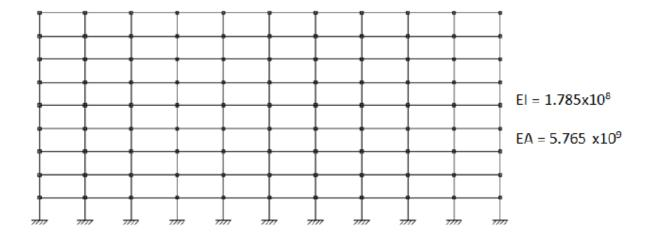
Shear deformations are excluded. Each beam/column is represented by one finite element. Consistent mass is assumed.
