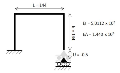
All elements are constant and equal El. Axial and shear deformations are ignored; to achieve the former analytically the cross sectional area was increased by a factor of 100,000 to make axial deformation negligible.
