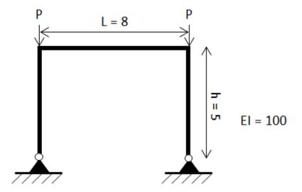
All elements are constant and equal El. Axial deformations are ignored; to achieve this the cross section area is set to 1000. The number of elements per member is varied between 0 and 5.
