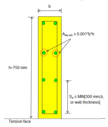
To control cracking in beams with a total depth > 750mm, side bars are provided in the side faces of the beam.  $^{1}$
