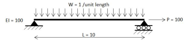
Shear deformations are excluded. Results are independent of cross section area; therefore any reasonable value can be used. The number of internal nodes varies from 0-9.
