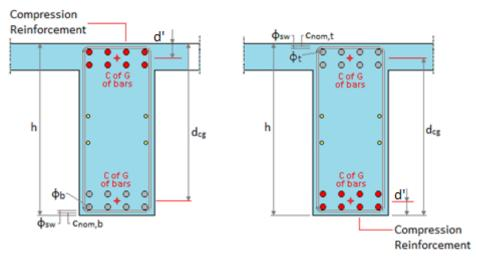
Tension Reinforcement in Bottom of Beam
