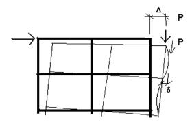
To obtain true design forces and moments, which accommodate all the P-Delta effects, then the analysis method used should account for both P- $\Delta$  and P- $\delta$ ; both the deltas ( $\Delta$  and  $\delta$ ) are inextricably linked – an increase in one brings about an increase in the other.
