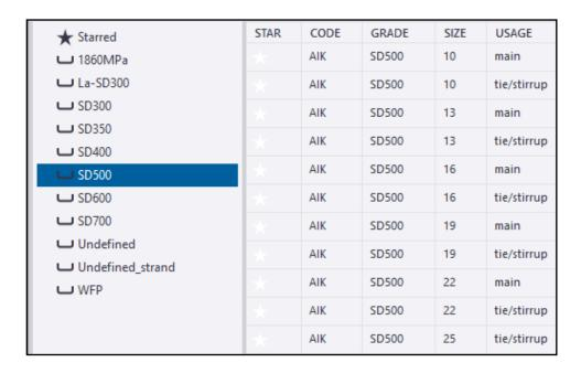
Once all of the entries have been completed, save the file and then change the extension to be '.cnv'. The file is then available for selection during the Rebar Grade Conversion phase by using the Rebar grade conversion file entry.
