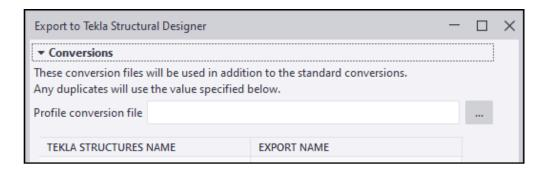
Entries where no conversion can take place will be marked as --- **NO MATCH** ---. The user will then need to identify the profiles which are not recognized and create a Profile Conversion file. This file should provide a recognized conversion for each of the unmatched profiles.
