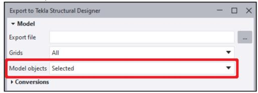
Please note that when using the option for **All** Model objects during the export process, this will include connections and other ancillary items which cannot be designed in Tekla Structural Designer.
